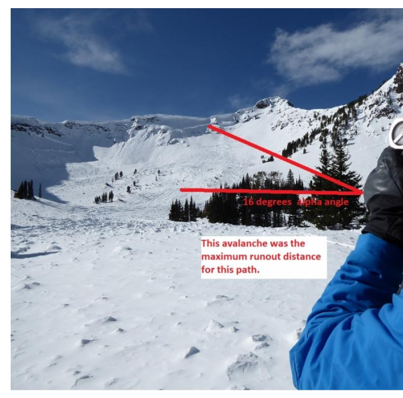
I measured the Alpha Angle (angle from crown to toe of debris) at 16 degrees. This is a very low angle that signifies the avalanche ran about as far as it ever could based on the size of the path. I took 5 measurements using 2 inclinometers to make sure this was correct. Photo: GNFAC
